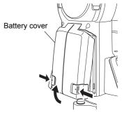
Insert the battery with the arrow shown on it downward while pressing toward the instrument.
