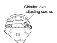
Adjust the adjusting screws until the tightening tension of the three screws is the same to align the bubble in the middle of the circle.
