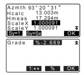
Press [OK] on the screen of step 11 to define the baseline. <Set-out line> is displayed. Move to settingline measurement.
