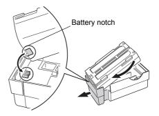
Slot the top end of the battery into the battery adapter. The extendable portion of the battery adapter will automatically retract and hold the battery in place.
