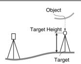
After inputting the target height, accurately sight the target.
