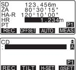
Check the input data, then press IREC1.
