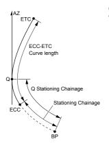
Calculation using BCC as reference: "ECC→ETC Calculation"
