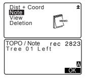
After inputting the note data, press [OK] to return to <TOPO>.
