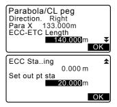
Press [OK] in the screen shown in step 5 to calculate the center peg coordinates. The coordinates are then displayed in this screen.
