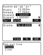
Press [1:\*\*] to change the grade display mode to "1: \* \* = elevation: horizontal distance".
