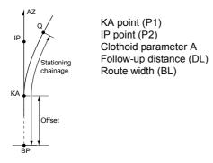
Calculation using arbitrary point between KA1 and KE1 as reference: "KA→KE Calculation 2"
