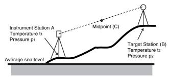
• If the weather correction is not required, set the ppm value to 0.
