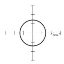
■ Target for Laser plummet adjustment
