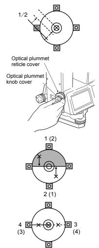
Check the adjustment by rotating the upper part of the instrument.
