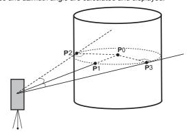
The azimuth angle of the center of the column is 1/2 of total azimuth angle of circumscription points (P2) and (P3).
