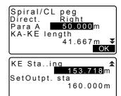
Press [OK] in the screen shown in step 5 to calculate the center peg coordinates. The coordinates are then displayed in this screen.
