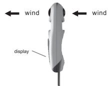
Point the Propeller towards the wind direction
