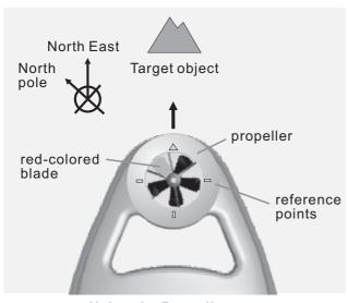
Using the Propeller as a Mechanical Compass
