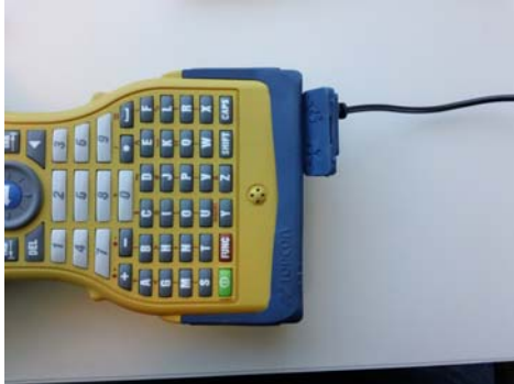
Figure 2-2. Charging the Batteries
